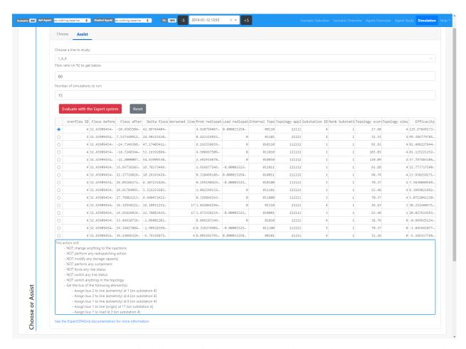
You can now see the results by simulating the action in the Compare section. The flow on  $1_4_4$  is now way below 80% but at the cost of a higher flow on adjacent lines and higher losses.
