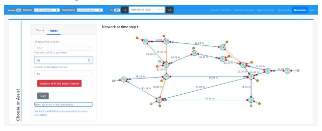
Evaluate the expert system and choose the first (i.e. best) action. It will reconfigure the substation 4 to make to flow on line 1\_4\_4 go below 80%.
